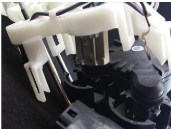
4 – remove the OE pump outlet spacers to be reused on the outlet of the DW300c pumps. The OE fuel sock can be reused, but will require trimming to fit the DW300c pumps
