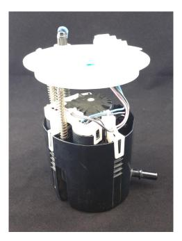
9 – reinstall the assembly into the fuel tank and attach a length of hose to the outlet of the pump assembly allowing it to drain into a fuel safe container and prime the fuel pump assembly
