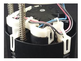
1 – separate the center section of the assembly from the bucket by lifting the three (x3) tabs around the perimeter. While separating the assembly use caution to not to kink or pull the small hose from the assembly (green circles), it is a small fitting and even a moderate force could cause it to break
