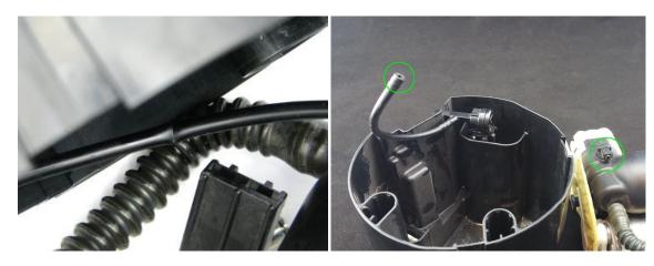
2 – remove the ground from the side of the assembly by pushing the tab (green circle) down and pulling the wire up
